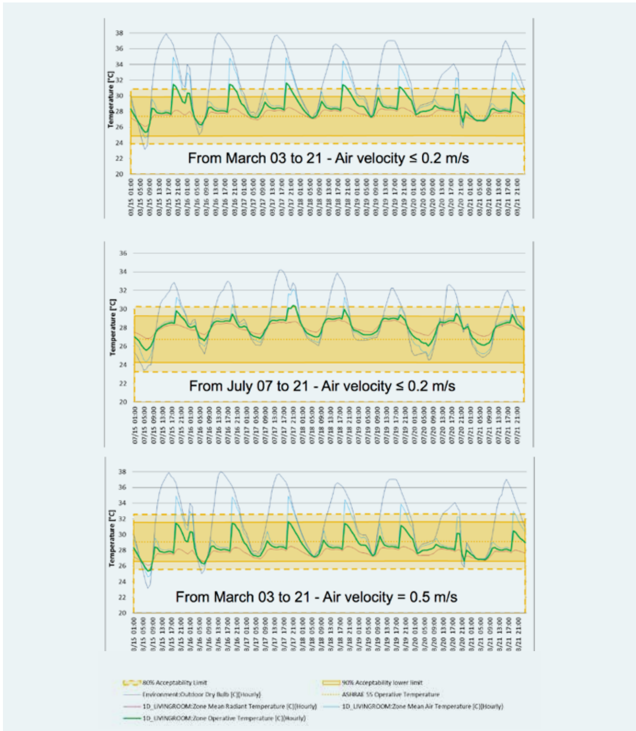
FIGURE A.5-11 LIVING ROOM HOURLY TEMPERATURES IN THE HOTTEST (03/15 TO 03/21) AND LEAST HOT (07/07 TO 07/21) PERIOD AND ASHRAE 55 ADAPTIVE COMFORT BAND FOR INDOOR AIR VELOCITY ≤ 0.2 M/S AND 0.5 M/S
