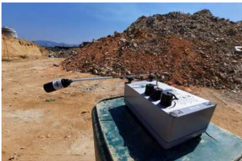
Osiris Environmental Particle Monitor Device / Bakalian Waste Storage Site / © UN Habitat 2021
