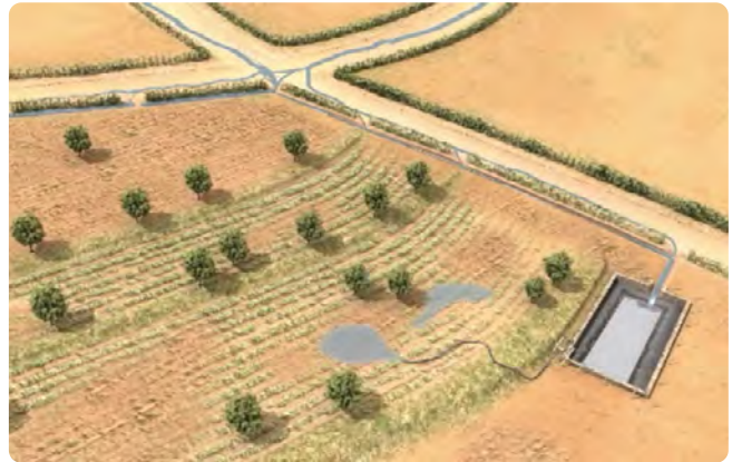
Figure 23 Example of concentrated road runoff harvesting by diverting flows into retention ditches or basins 34
