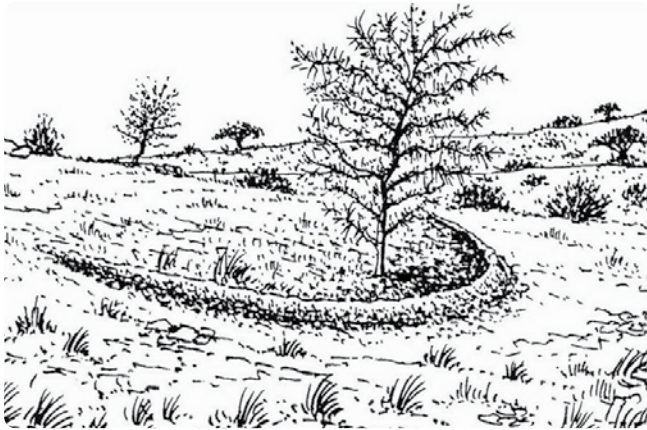
Figure 73 Semi-circular bunds used to retain water for trees 105
