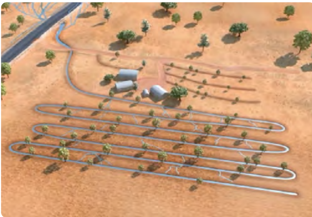
Figure 22 Example of concentrated road runoff harvesting by diverting flows into retention ditches or basins 33
