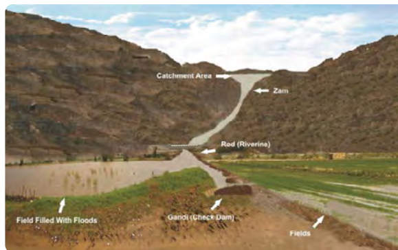
Figure 12 Schematic diagram of floodwater, from the mountains to the fields 2
