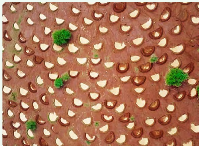
Figure 77 Bunds implemented by Justdiggit in Kuku, Kenya
