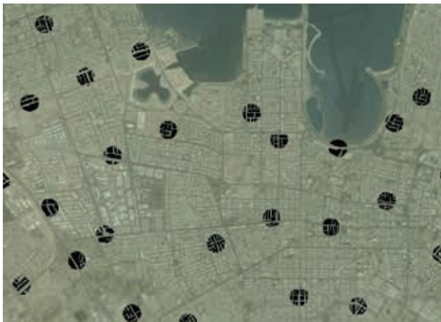
Figure 2: Halton sequence of coordinates used to select sample of locales in an urban area
